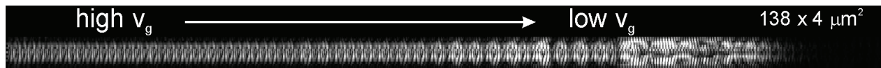
A near-field image of light propagating from left to right in a chirped waveguide.
